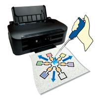
Just inkjet it: Inkjet printing plays an important role as a process technology in the fast-growing field of microfluidic devices made of paper. This Review introduces the basics, strengths, and weaknesses related to the inkjet printing of functional materials essential for paper-based analytical devices. The discussion includes fundamental aspects as well as examples of analytical applications.
